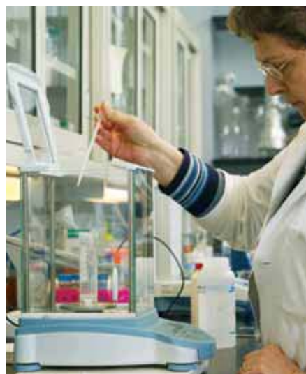
Removable front, side and back glass panels
