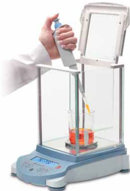
Hinged top and sliding side doors allow easy access
