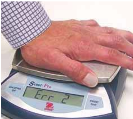
Mechanical and software overload protection
