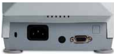
MB25/23 RS232 interface connection
